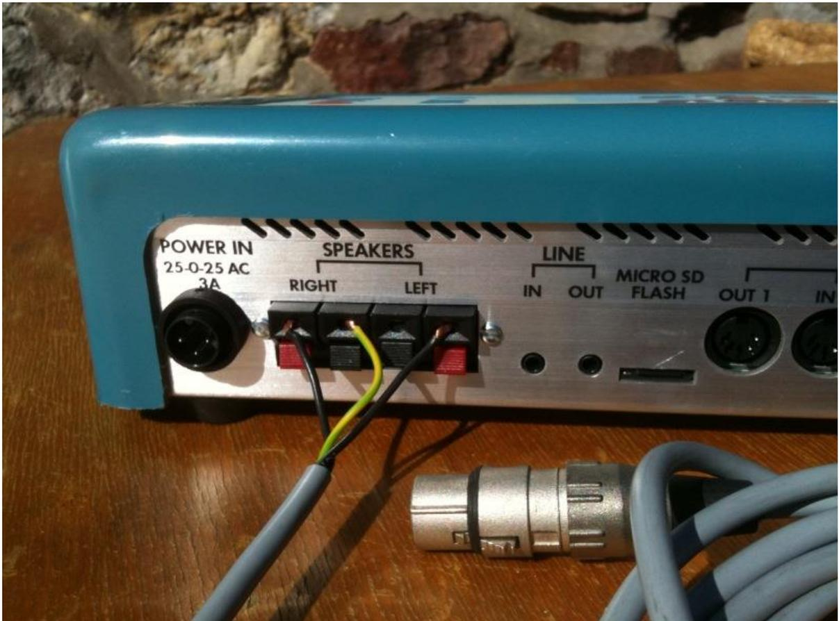
5. Switch on the power supply to your amplifier or Soundbeam 5. If using an MP3 player/ipad/smartphone or CD connect the chosen device to the amplifier using the headphone socket or line out of your device to a line in on your amplifier or line in on the Soundbeam 5.
